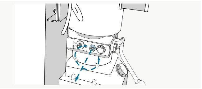
To change the lift capacity, open or close the lift capacity valve on the motor. Tighten = more pressure = more lifting power. When opening, pressure is released from the system and the lift would lift with less lifting force.
