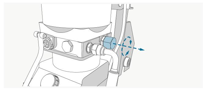
To change the descension rate, the descent valve must be opened or closed. In order to lower the stage more quickly, the valve must be opened.
