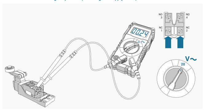
To do this, switch the multimeter to 20 V direct current. If the cable leading to the limit switch works, the multimeter shows how many volts are running through (it should be 24 V). If this is not the case, the plug connections on the control panel and limit switch must be checked, or the cable must be replaced.
