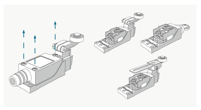
To test the current flow, first unscrew the cover of the given limit switch.
