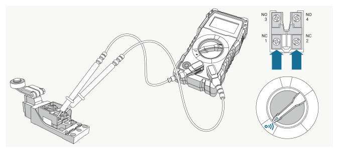
You will need a multimeter for this process. Switch it to signal - flow and hold the two diodes to the screws of connectors NC-1 and NC-2. If the limit switch is working correctly, the multimeter should beep. If the multimeter does not produce a beep, the limit switch must be replaced.
