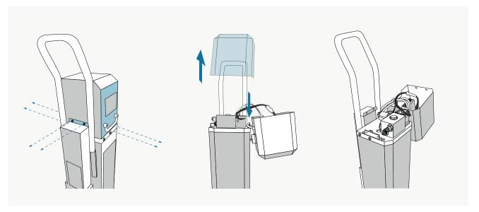
Loosen the screws on the side of the control panel and carefully loosen the cover. Hook the cover sideways into the control panel to have open access to the required screws.
