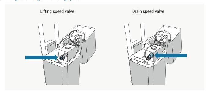
To increase the lifting speed, you have to turn the lower screw counterclockwise (clockwise to raise the platform more slowly). To increase the descent speed you need to turn the top screw counterclockwise (clockwise to slow down the stage).
