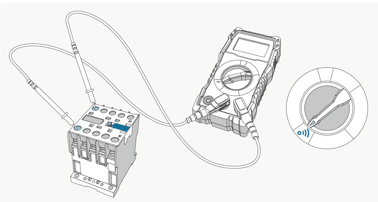
You need a multimeter to test the function. To do this, plug the diodes into the opposite phase inputs and outputs and turn on the main switch. When current passes through, a sound should be produced.
