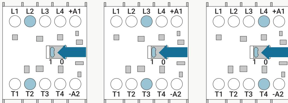
Repeat the process for all phases. Phase input is row L1 and phase output is row T1. Please do not connect the control panel to the mains at this point! If there is no tone from the multimeter on any phase, the motor protector needs to be replaced.
