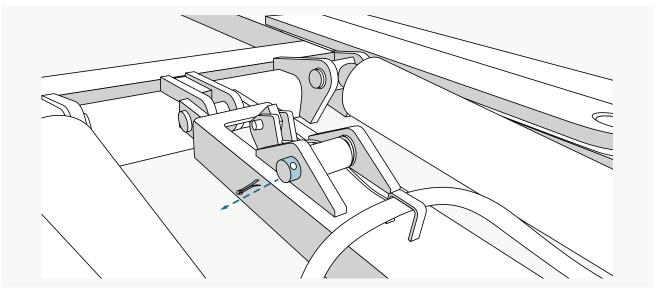
Using pliers, fold over the ends of the locking ring and pull it out of the notch.
