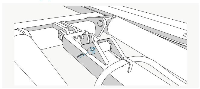
Replace the locking ring and unfold the ends with pliers to re-secure the bolt.
