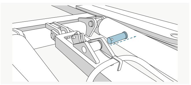
Remove the bolt to expose the tension spring and safety catch.
