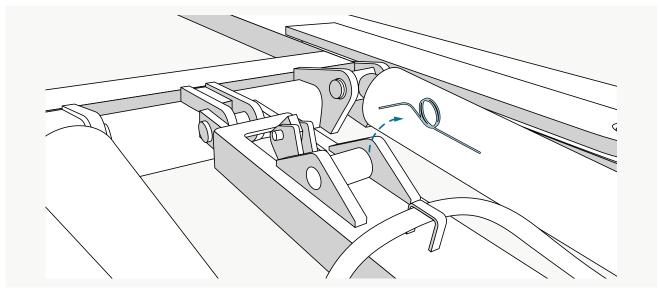
Now remove the defective tension spring.
