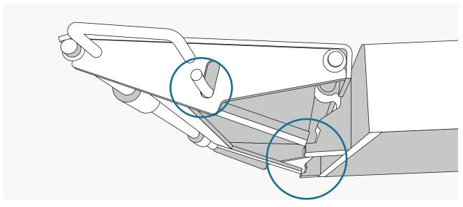
The ramp no longer engages properly due to the bent latch handle.
