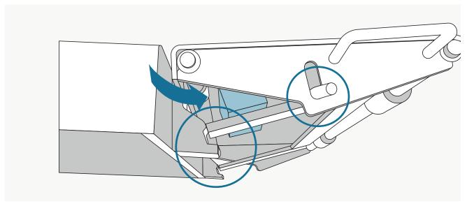
In the event that the handle is bent downwards, you must block the handles from below before folding the ramp down to avoid material damage. A block of wood or something similar works best.
