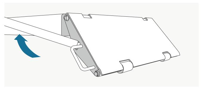
Fold in the catch of the drive-on ramps and let the ramp hang. Bend the handle to its original position - In this case, use a steel pipe to bend it up.
