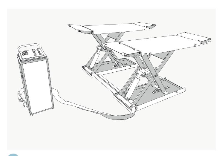
**Problem**: The access ramps of the lift are not level with the platforms.
