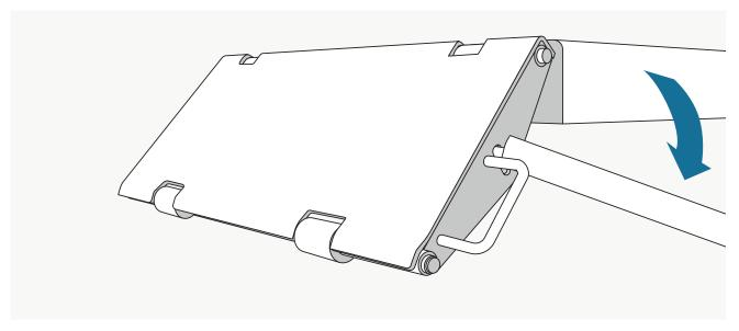
Fold in the catch of the drive-on ramps and let the ramp hang. Bend the handle to its original position - In this case, use a steel pipe to bend it down.
