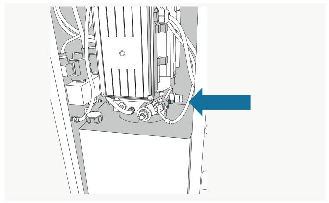
The smaller valve (throttle valve) on the right side inside the control panel is responsible for the lifting power. If you turn it off, you lift with more lifting power, if you turn it on, you lift with less lifting power.
