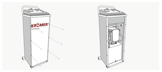
Open the control panel by loosening the screws.
