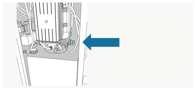
Open or turn the large red valve to control the rate of descent. Open means the stage has a faster descent rate, closing the valve means the descent rate decreases
